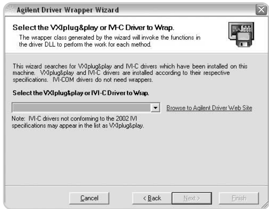
Figure 11. Agilent's IVI-C Driver Wrapper Wizard makes it easy to use IVI-C compliant drivers in VS .NET.
